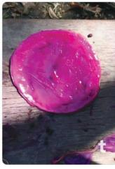
**Figure 2.** Growing and dyeing microbial cellulose. The fabric is grown from SCOBY culture, dyed with plant pigments found on the farm, such as Malabar Spinach berries, shown here, turmeric and chili powder. The fabric dries to a leather-like textyure.
